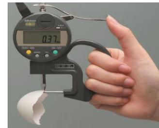
Shell Thickness Micrometer
